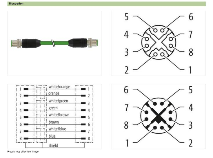
Cable length 45 m Side 1 0,6 Nm Tightening torque Mounting method inserted, screwed Coating contact gold plated
